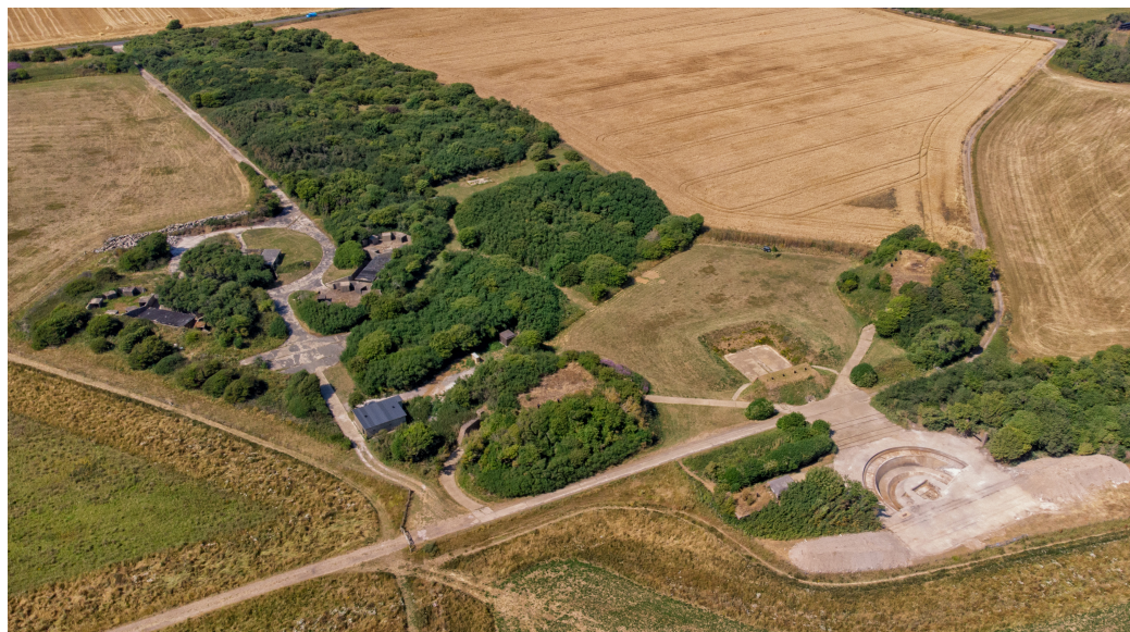
View north over the 15-inch Wanstone Battery: the recently excavated emplacement (bottom right) of 'Jane'; two covered magazines (centre and centre-right); the Crew Shelter, built below ground and with bund protection (centre right). At left is the D2 Heavy Anti-Aircraft Site, for four 3.7-inch guns in hexagonal emplacements, serviced with two magazines (© National Trust)
